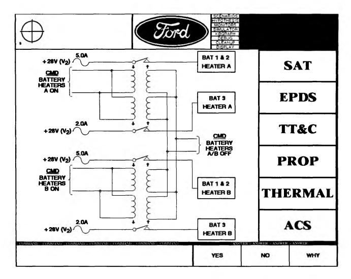
operation of the system. These screens show portions of the system's model of the satellite and its subsystems. The use of frames to build the system's models allowed the designers to organize them so that the knowledge could be easily accessible and comprehensible to both diagnostic experts and satellite operators.
